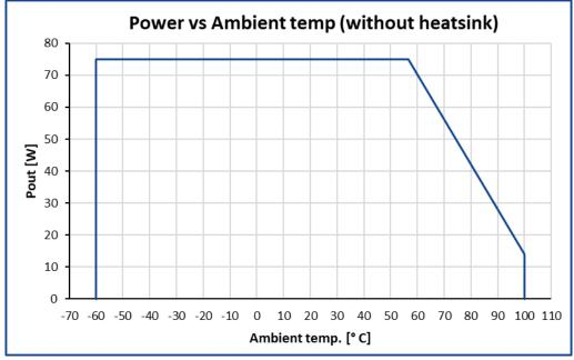
Power vs Ambient temp. graph is given for short-term use cases. To use the units without a heatsink it's mandatory to consult with the manufacturer.
