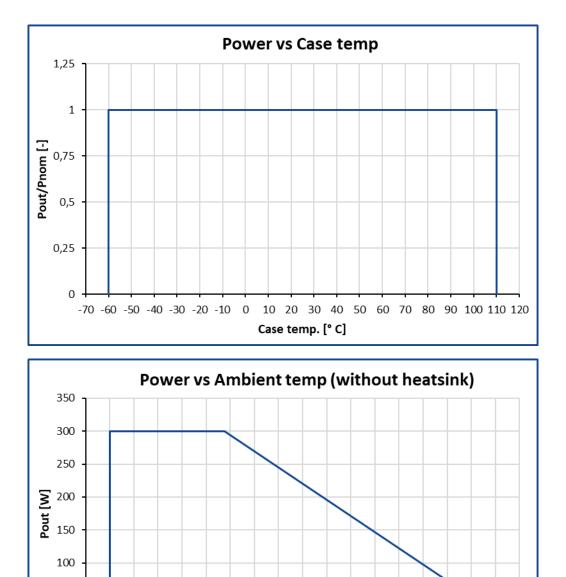
Power vs Ambient temp. graph is given for short-term use cases. To use the units without a heatsink it's mandatory to consult with the manufacturer.
