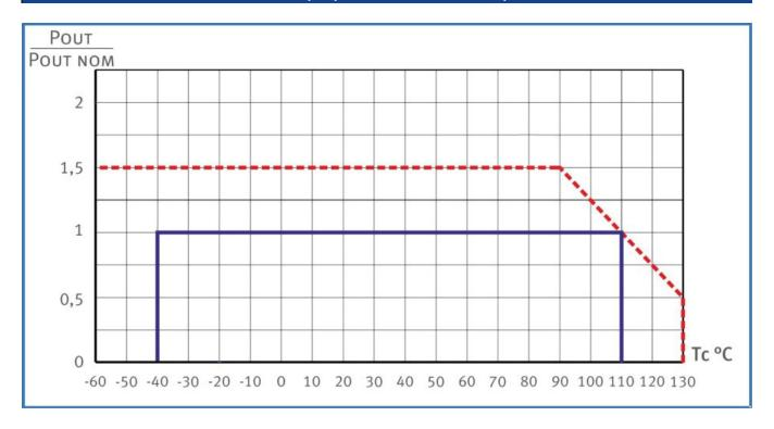
\_\_\_\_\_ Standard maximum power output based on case temperature.
